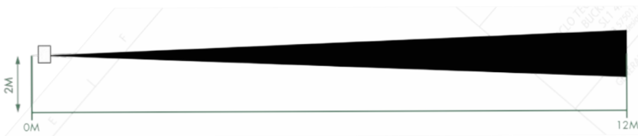
Typical field of view diagram when used in conjunction with Type A, B
